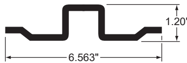
SIDE POST, A-SLOT, STEEL, 128"
